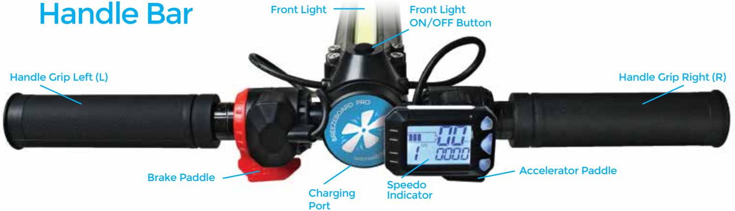
Once charged, its time to get accustomed with the simple controls on your Breezeboard PRO Electric Scooter. First, press the large middle ON/OFF button on the **Speedo Indicator**, this button will turn on and turn off your scooter.
